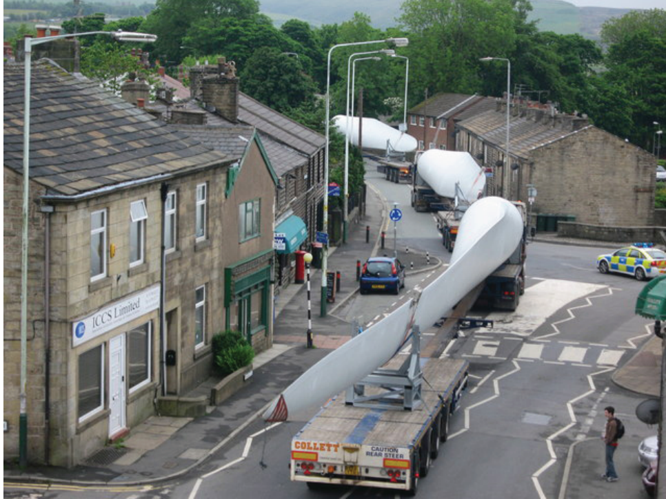
Figure 1: A convoy of wind turbine blades passing through the village of Edenfield, England. Photo Credit: Anderson (2007)
