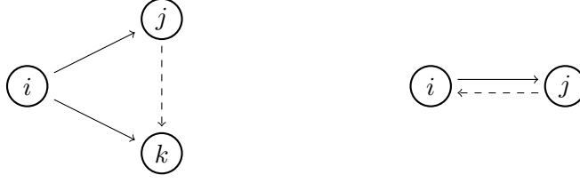
Figure 7: Networks from Sections 4.2 and 4.3. The left panel adds a correlating link. The right panel adds a backward link.
